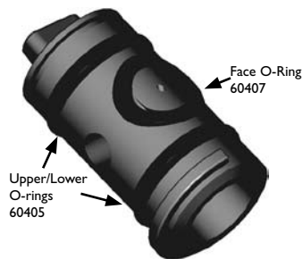
Figure 25b - Nozzle Valve Plug
