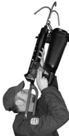
Figure 21b - Angle for Vertical Deployment
